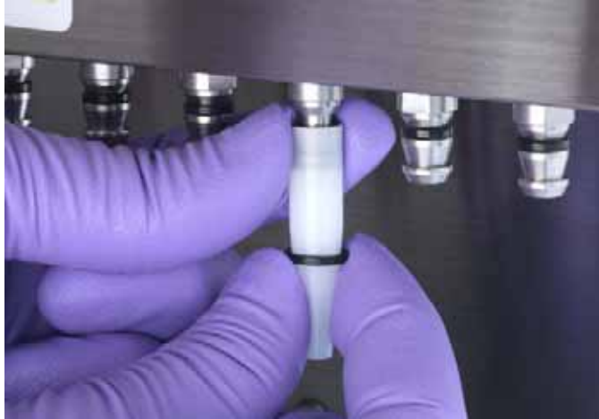
Figure 3.9 Replacing the D-ring
